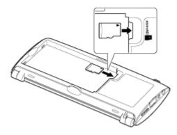
4. Carefully slide the microSD memory card into the slot until it clicks into place.
